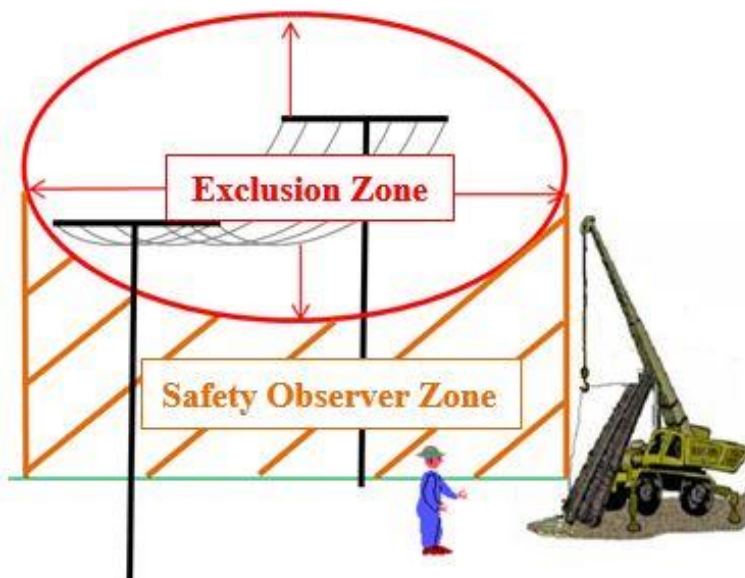
Figure 2: Top view of Safety Observer Zone for slewing cranes
