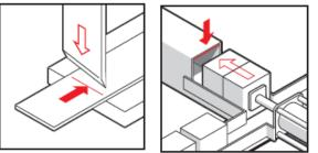
Figure 7 – Sliding hazards diagram
