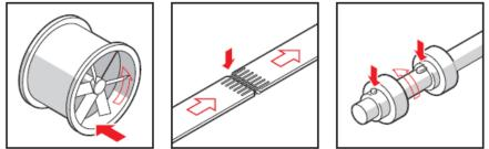
Figure 4 – trapping hazards diagram
