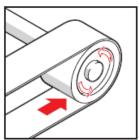
Figure 2 – Trapping hazards diagram
