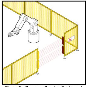
Figure 2 – Presence Sensing Equipment
