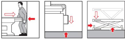
Figure 11 – Crushing hazards diagram
