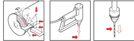
Figure 10 – Puncturing hazards diagram
