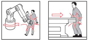
Figure 9 – Impact hazards diagram
