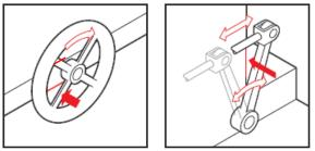
Figure 6 – Shearing hazards diagram
